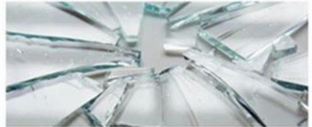
Normal glass broken into big and sharp fragments easy hurt human
