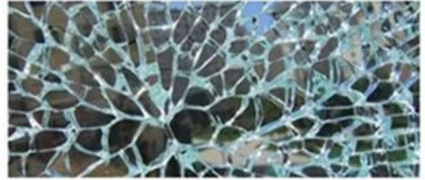
Toughened glass broken into small cubical fragments high safety human harmless
