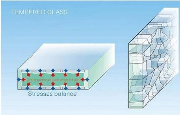
The comparison between tempered glass, heart strengthened glass and normal glass
