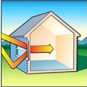
Standard clear unit Conventional aluminum spacer Air Fill SHGC – 0.75
