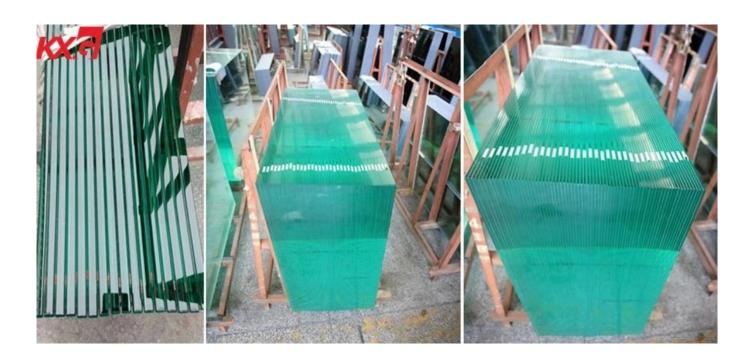
12mm <u>clear Semi-tempered glass</u>, also known as 12mm colorless heat-strengthened glass, it is a kind of heat processed glass that naturally cooled after tempered heating the 12mm clear float annealed glass, to obtain half toughened glass which strength better than annealed glass, while avoid self-explosion phenomenon.
