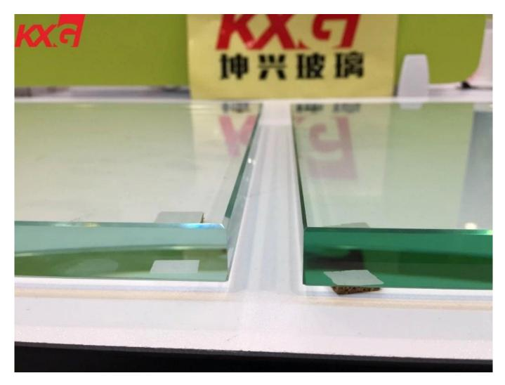
Difference between 15mm low iron toughened float glass and 15mm ordinary clear toughened float glass.
