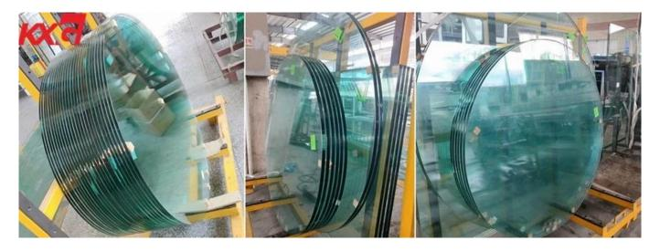
Toughened glass is fabricated by heating annealed glass to over 600°C and cooling it rapidly, which locks the outer surfaces of the glass in a state of high compression, and the core or center of the glass in compensating tension. Round <u>clear toughened glass</u> is widely used for table top or center table etc.
