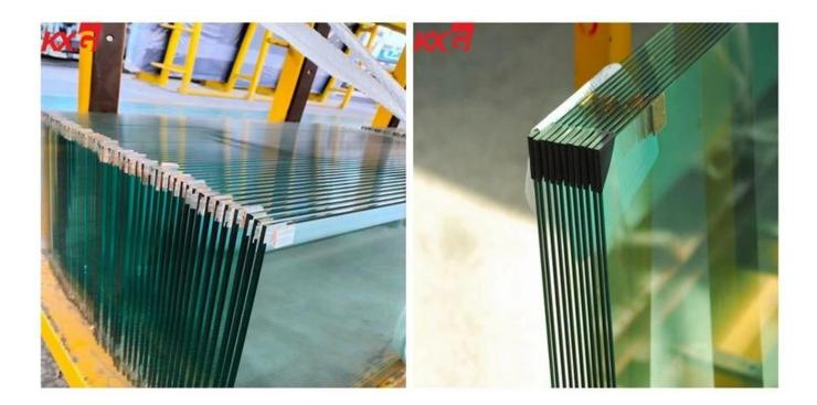
For the\_shower door glass / shower enclosure glass can be flat shape or curve shape, could be tempered or laminated, can been drilling holes, notches ,cut out precisely to install the fittings, as per your design drawing. The shower glass thickness normally is 4-10mm, and 5mm, 6mm,8mm is more popular by the market.
