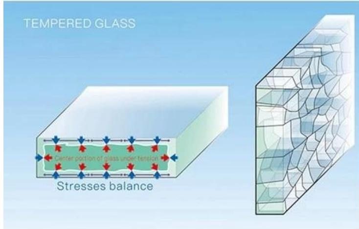
Toughened glass broken into small cubical fragments high safety human harmless.
