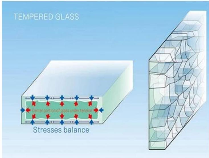
Toughened glass broken into small cubical fragments
