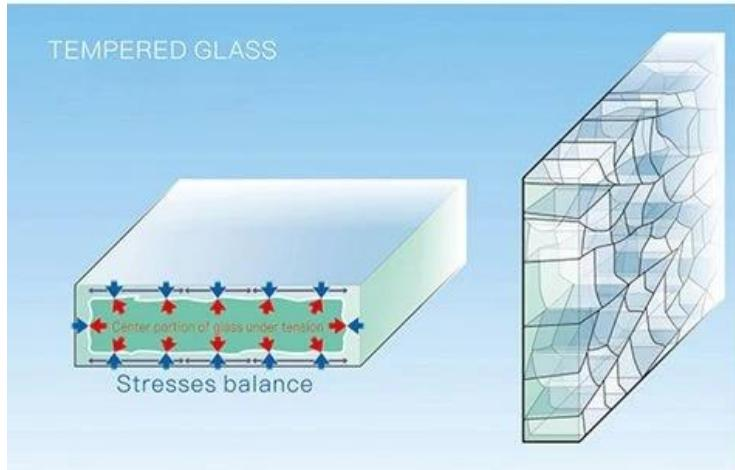
Toughened glass broken into small cubical fragments
