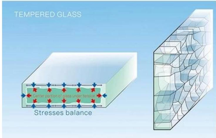
Toughened glass broken into small cubical fragments
