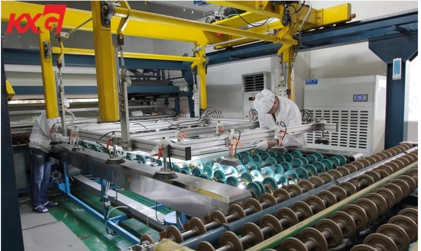
6 mm +0.76 mm PVB + 6 mm malinaw na ulo laminating glass stay autoclave 8 oras
