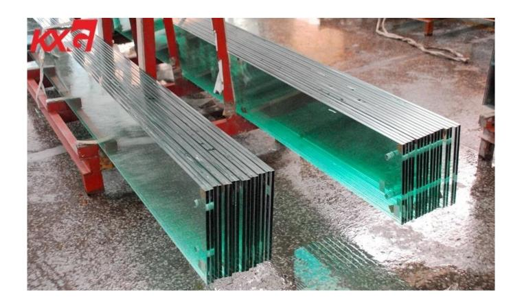
21.52mm SGP Tempered Laminated Glass
