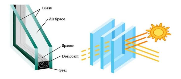
In addition, insulating glass can effectively insulate sound. Due to the spacing between glass panels, insulating glass can reduce the transmission of external noise and create a quiet and comfortable indoor environment. Especially suitable for noisy urban environments or places where privacy needs to be protected.
