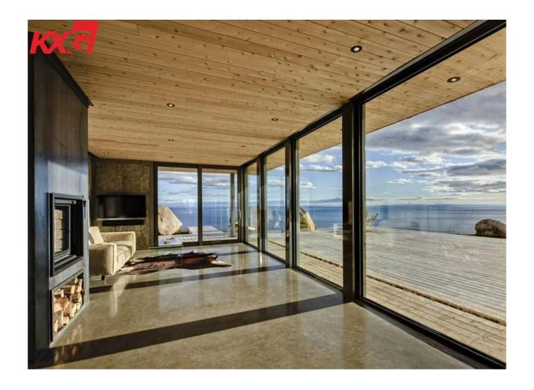
8mm clear tempered glass+6 Air space+8mm clear toughened glass doors and curtain wall
