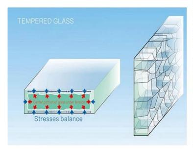
Toughened glass broken into small cubical fragments high safety human harmless.
