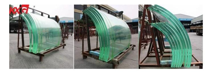
About 8.76mm Colorless **Tempered Laminated Glass** 8.76mm Clear Tempered Laminated Glass is made up of two pieces 4mm clear toughened glass permanently bonded together with 0.76mm PVB interlayer via a controlled, highly pressurized and industrial heating process. The lamination process results in the glass panels holding together in the event of breakage, reducing the risk of harm. Laminated Glass is classified as Grade A Safety Glass.
