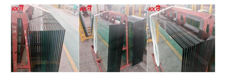
Due to 12mm heat soaked testing glass is made by increasing the temperature of 12mm tempered glass up to 290°C±10°C so heat soaked tested glass also have the same characteristics and advantages of tempered glass.
