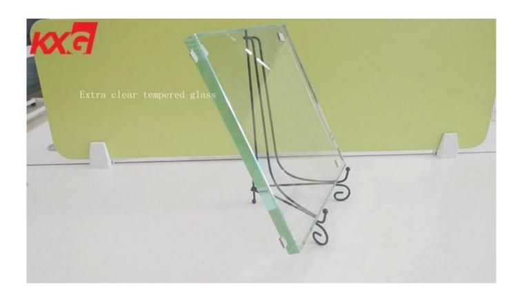
19mm extra clear tempered glass,19mm ultra clear toughened glass, 19mm super transparent tempered glass, it is deep processed by 19mm ultra clear float glass, one of the safety decorative glass, shape available in flat and curved. Compare with 19mm clear tempered glass it with high visible transmittance, widely used for high level area such as hotel tabletop, jewelry storefront, fish tank, balustrade, etc.
