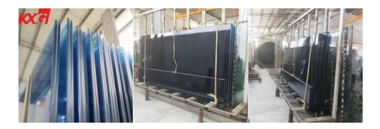
11.52mm light blue laminated glass, 554 ford blue laminated glass, light blue sandwich glass, it is made by 2pcs of 5mm transparent glass bonded together with 1.52mm ford blue PVB interlayer, is a kind of **safety glass**, decorative glass, heat control glass, high precise flatness, cut into size 11.52mm ford blue laminated glass, used for glass window, glass balcony, glass balustrade, glass partition.
