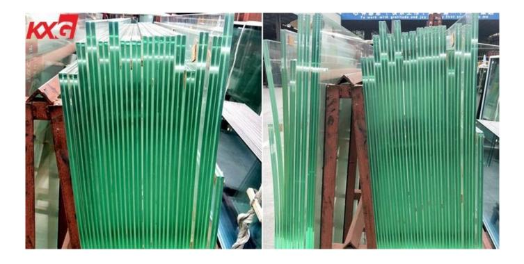
Building 12.76mm **laminated Glass** which made by two pieces of 6mm float glass bonding together with a layer or more and more adhesive film to make, its popular for office door, shop front door,etc. There's various design and pattern for choose as per required.
