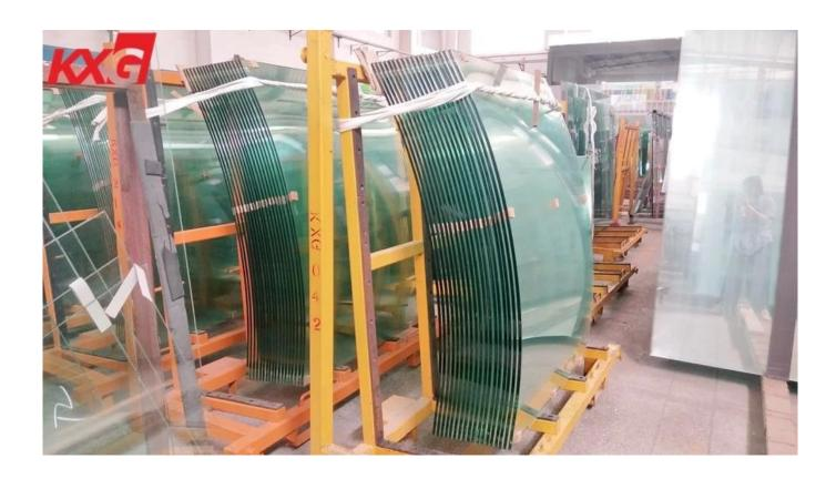
10mm clear curved tempered glass is shaped by dies controlled by computer, rapidly and uniformly cooled immediately after it is heated to the designed shape. This kind of glass has all the good performance of 10mm flat tempered glass, but has a higher intensity for the wind pressure and bending than the flat tempered glass.
