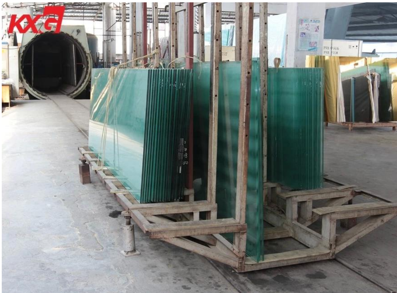
6mm+0.76mm PVB+6mm clear tempered laminating glass stay autoclave 8 hours
