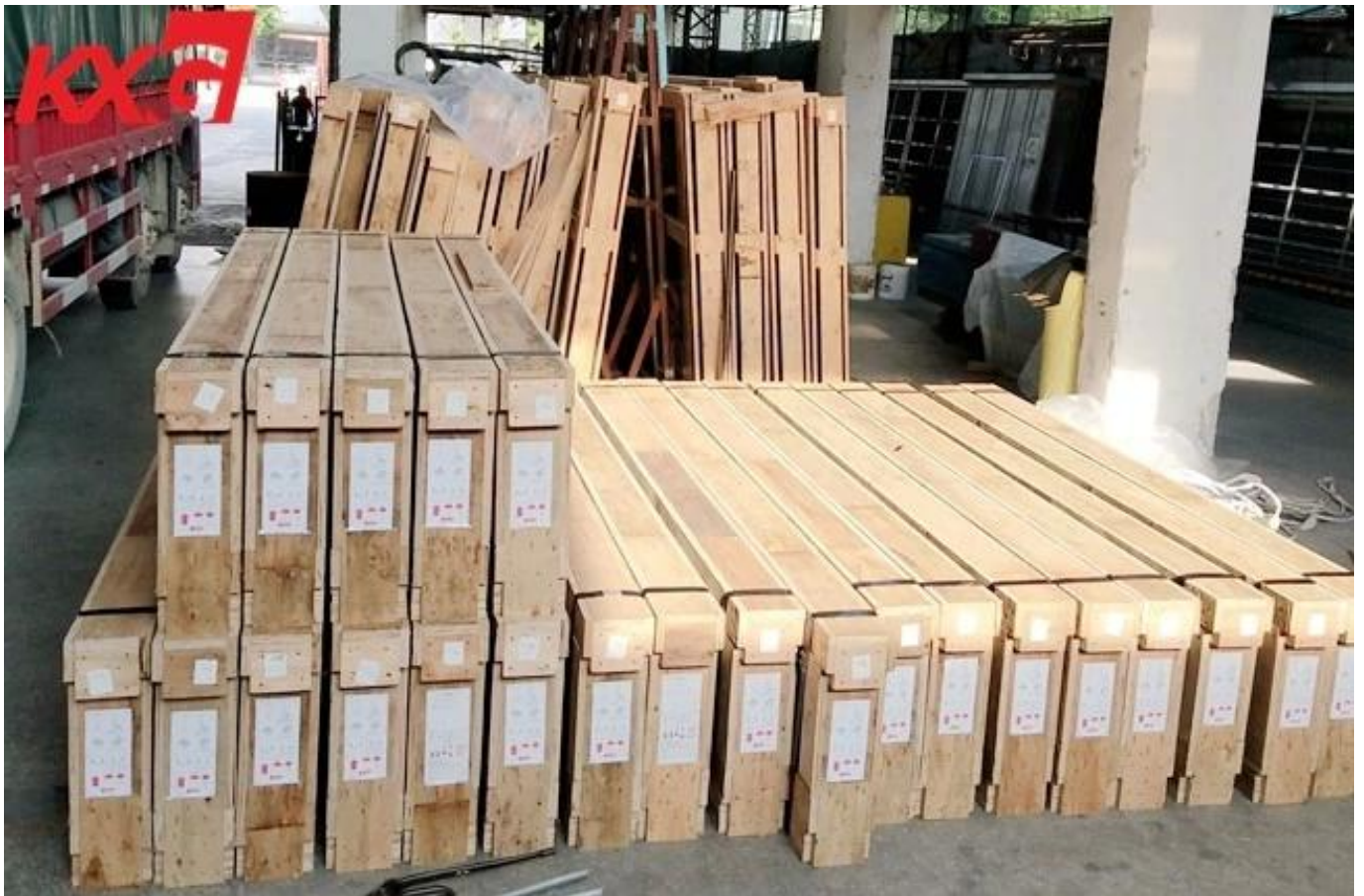
12mm low iron tempered glass packaging by plywood crate with steel belt
