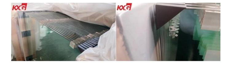
1. 12mm clear tempered glass, it is stronger 4 to 5 times than 12mm float glass.
