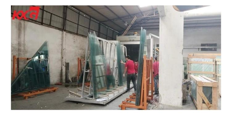
11.52mm clear toughened laminated glass heat soak test equipment at <u>Kunxing building gl</u> ass factory
