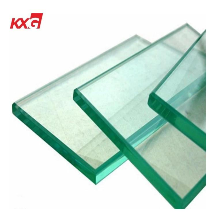
Heat soak tested, HST, which is also called hot-dipping test or igniting test, refers to the method of re-heat-treatment after armoring, it is a method to avoid self-explosion effectively, which is a pane of toughened glass is subjected to temperatures of 280° for several hours over a specific temperature gradient, to induce fracture.
