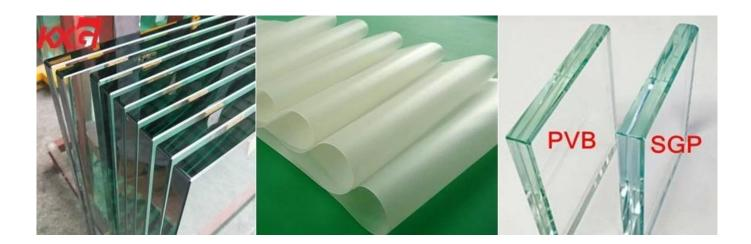
Excellent quality 15mm+1.52mm PVB/SGP interlayer+15mm <u>tempered laminated glass</u>, which is processed by 2pcs of 15mm clear or ultra clear or colored tempered glass with 1.52mm PVB interlayer or SGP interlayer to bond it. Which is a type of safety glass that holds together when shattered, widely used to the places where is the possibility of human impact or the glass could fall if shattered, like balustrade, skylight, storefront, floor, etc.
