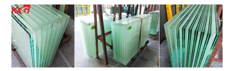
The 17.52mm frosted translucent **tempered laminated glass** can be made by two compositions, one is made by one piece 8mm frosted tempered glass and one piece 8mm clear toughened glass, with 1.52mm colorless PVB interlayer. The other composition is two pieces 8mm colorless tempered glass with 0.38mm frosted PVB and 1.14mm clear PVB interlayer.
