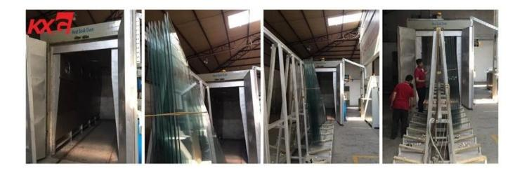
Heat soak testing after tempered glass manufacturing may destroy some defective glass sheets, but this procedure doesnot guarantee 100% elimination of nickel sulfide inclusions. In addition, the Heat soak process may increase cost, cycle time and scrap rate. Heat soak tempered laminated glass, made of two tempered glass by Heat soak test bonding and sandwich of PVB film or SGP film. It can be flat or curved.
