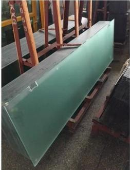
Laminated glass is actually two pieces of glass stuck to a thin intermediate layer. If it is damaged, the glass remains intact as each piece remains stuck to the central layer.
