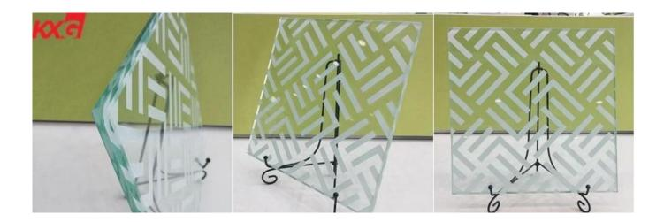
Silkscreen printing building glass is printing the need design or coloured on the glass surface with inorganic glazed which has high temperature resistance. After processed of drying and agglomeration, the silkscreen pattern design will be agglomerated permanently on the glass surface. Then via a thermal tempering process, to made for silkscreen printed tempered glass.
