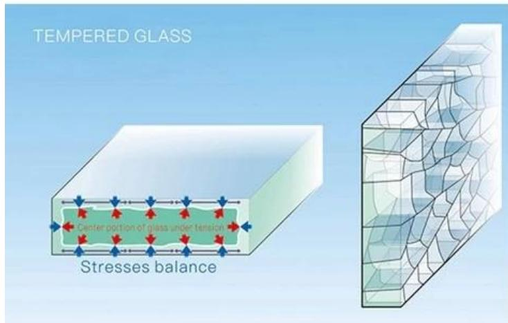
Toughened glass broken into small cubical fragments
