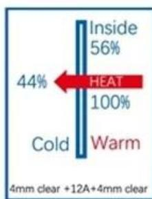
Insulated glass unit reduce heat loss by up to 56%
