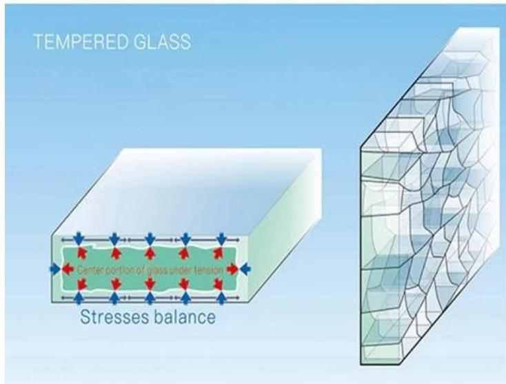
Toughened glass broken into small cubical fragments
