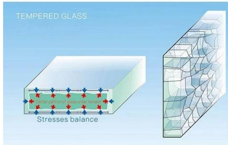
Toughened glass broken into small cubical fragments
